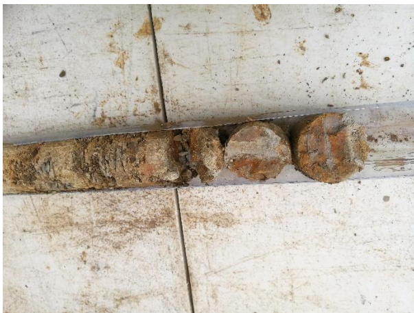
Photo 1. Clays and weathered shale were predominantly found on site
